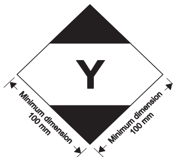
Mark for packages containing limited quantities conforming to Part 3, Chapter 4 of the ICAO Technical Instructions
